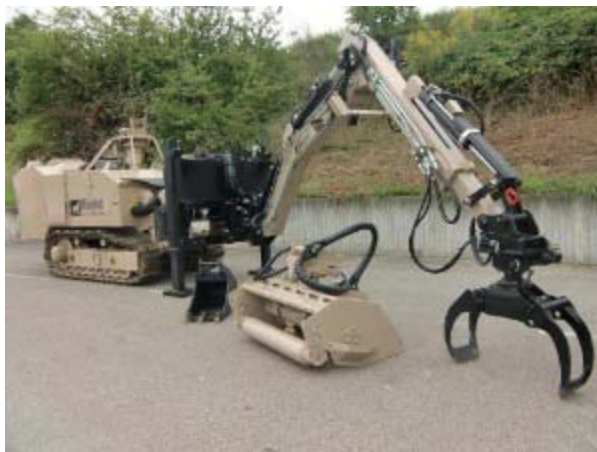
Remote controlled Mini MineWolf with robotic arm attachment for IED clearance (Photo: Business Wire)
